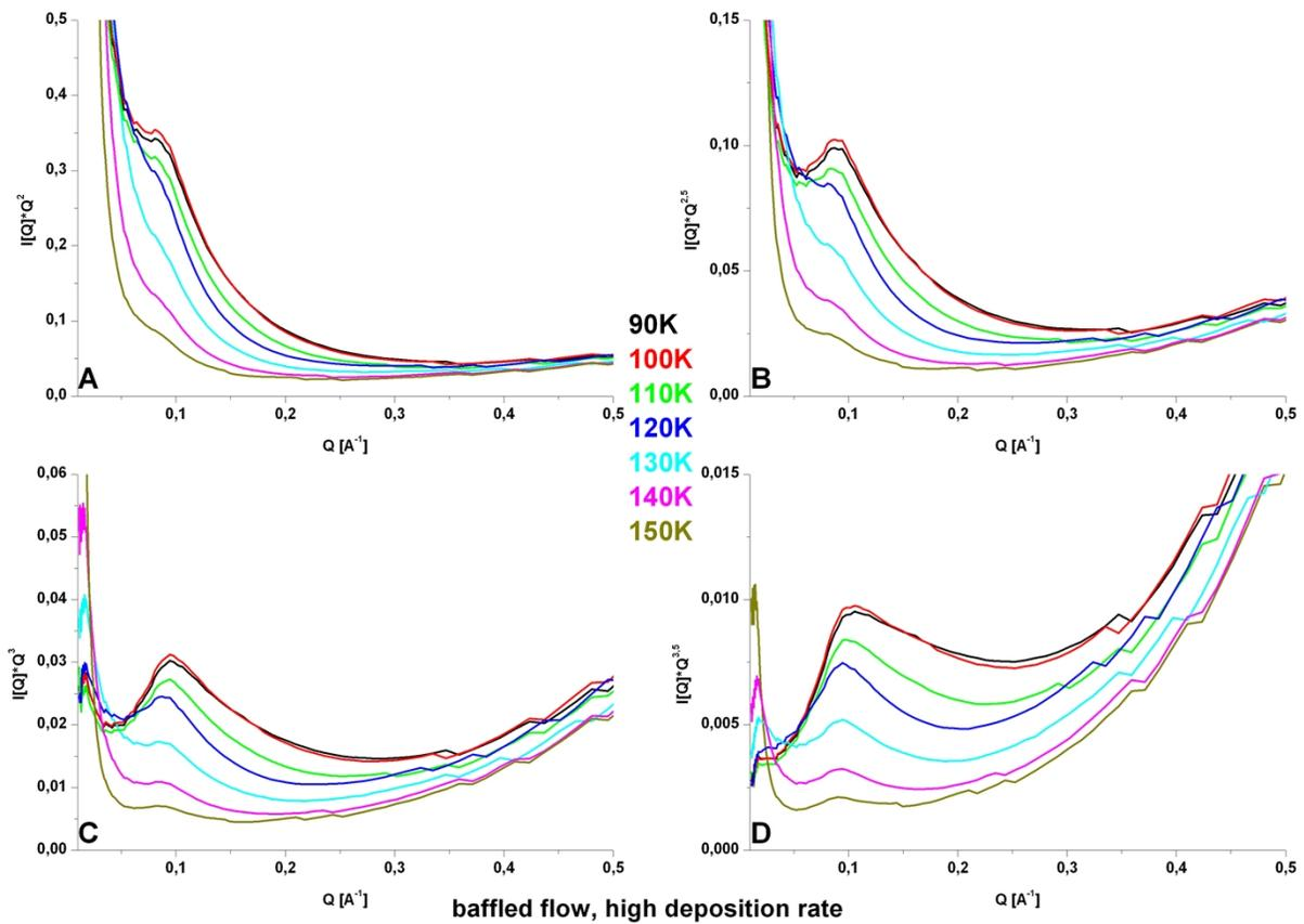
**Temperature evolution between 90 and 150 K of standard linear plots  $I(Q) \cdot Q^d$  versus  $Q$  with  $d$  between 2 and 3,5 for the baffled flow, high deposition rate sample.**
