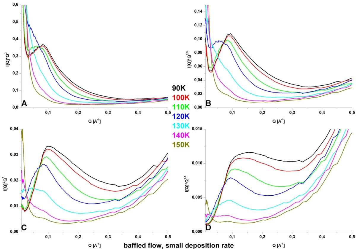
**Temperature evolution between 90 and 150 K of standard linear plots  $I(Q)*Q^d$  versus  $Q$  with  $d$  between 2 and 3,5 for the baffled flow, small deposition rate sample.**
