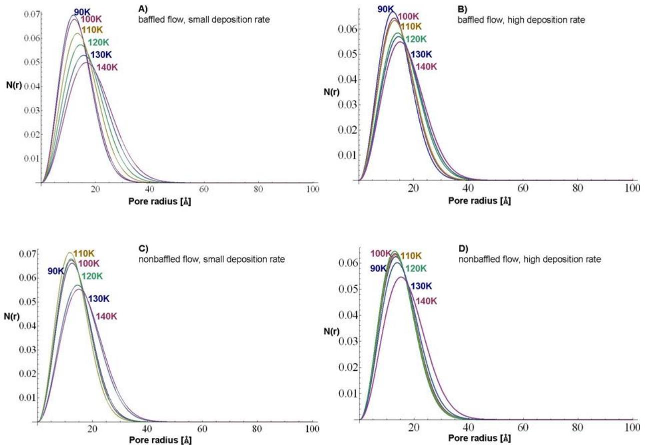
**Temperature evolution between 90 and 140 K of Maxwell pore size distribution for spherical pore shape**
